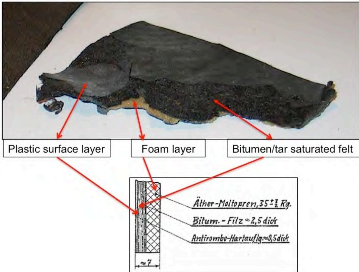
In addition to the foam-backed material, Mercedes also used another material with jute backing. Neither one proved to be very durable and long-lasting.
