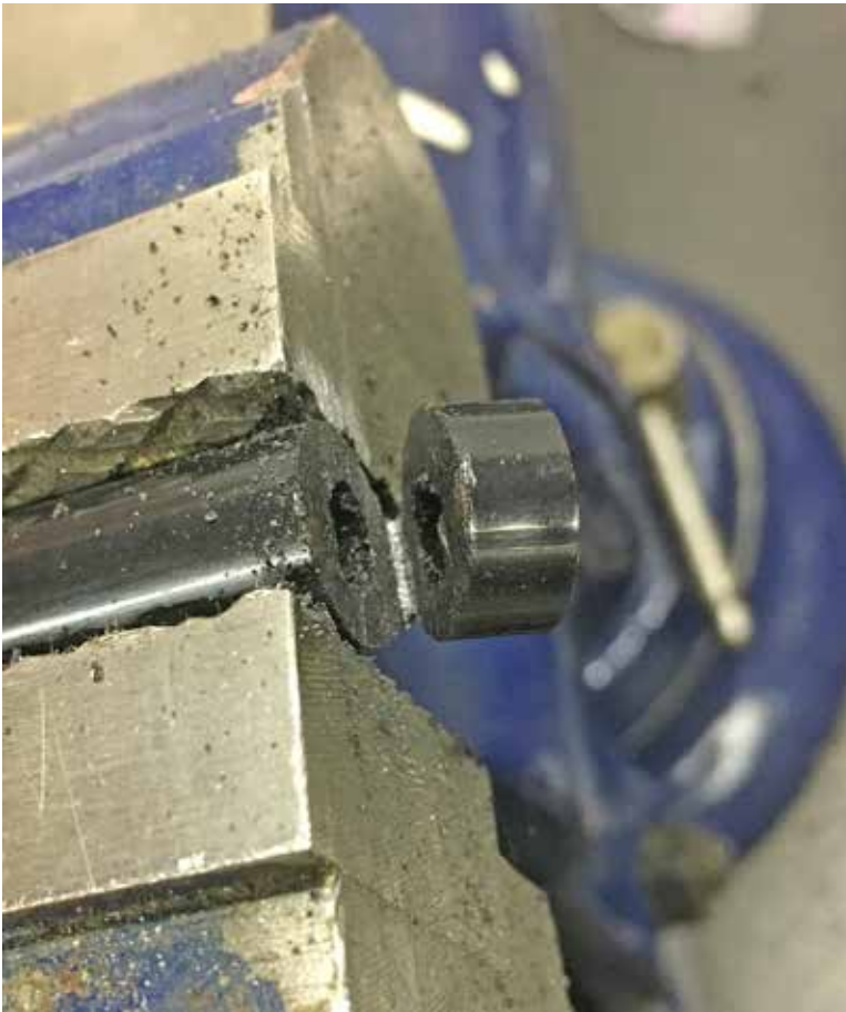
Photo immediately to the left shows the spacer cut.
