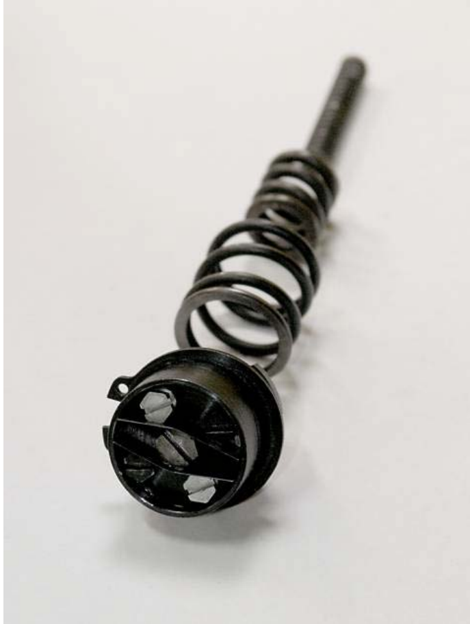
The adjusting screws: In the middle the idle screw, which is also accessible from the outside. The light ones for the upper, the dark ones for the lower partial load.
