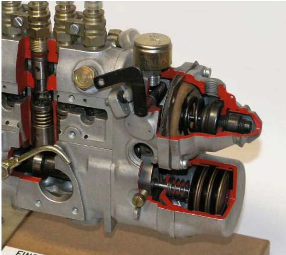
Sectional model with a clear view of the vacuum control (top right), below the regulation for air temperature
