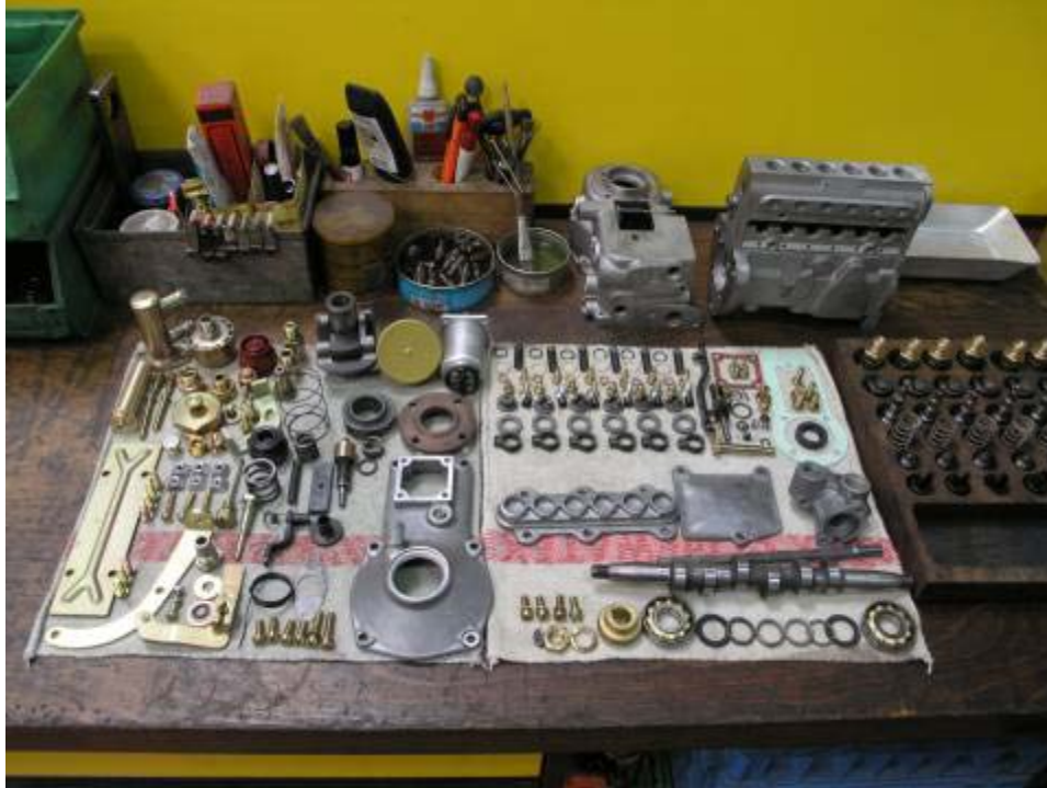
A completely disassembled six-piston pump
