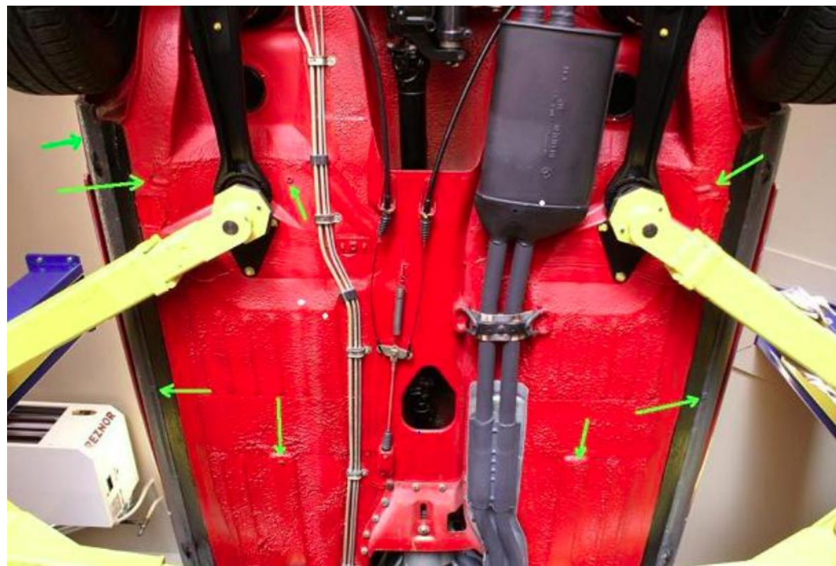
Box section drain
